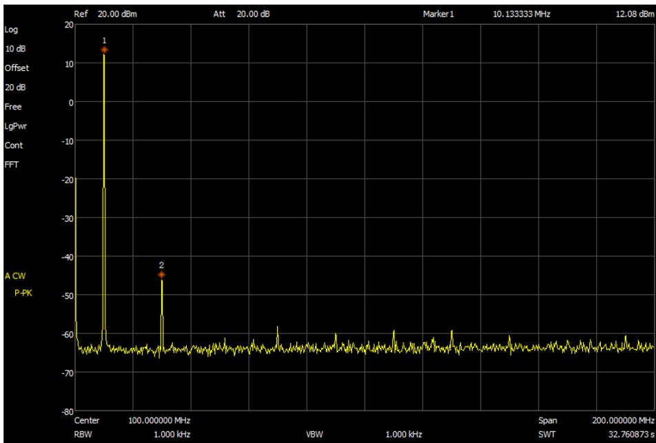
Figure 7.b ~ The PLL-GNSSDO output spectra is very clean with only the fundamental and 3<sup>rd</sup> harmonic (30 MHz) visible. The 3<sup>rd</sup> harmonic level is -58 dBc.
