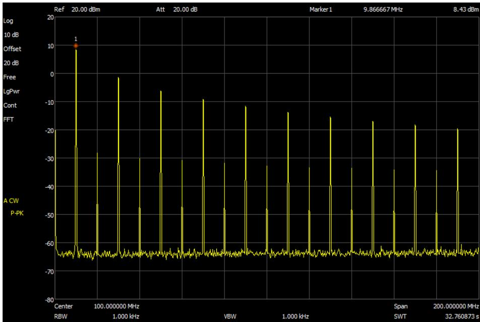
Figure 6.b ~ The MPGPSRC output spectra indicates an offset squarewave with harmonics spaced at 10 MHz intervals. The strongest harmonic is the 3<sup>rd</sup> harmonic (30 MHz) at -10 dBc.
