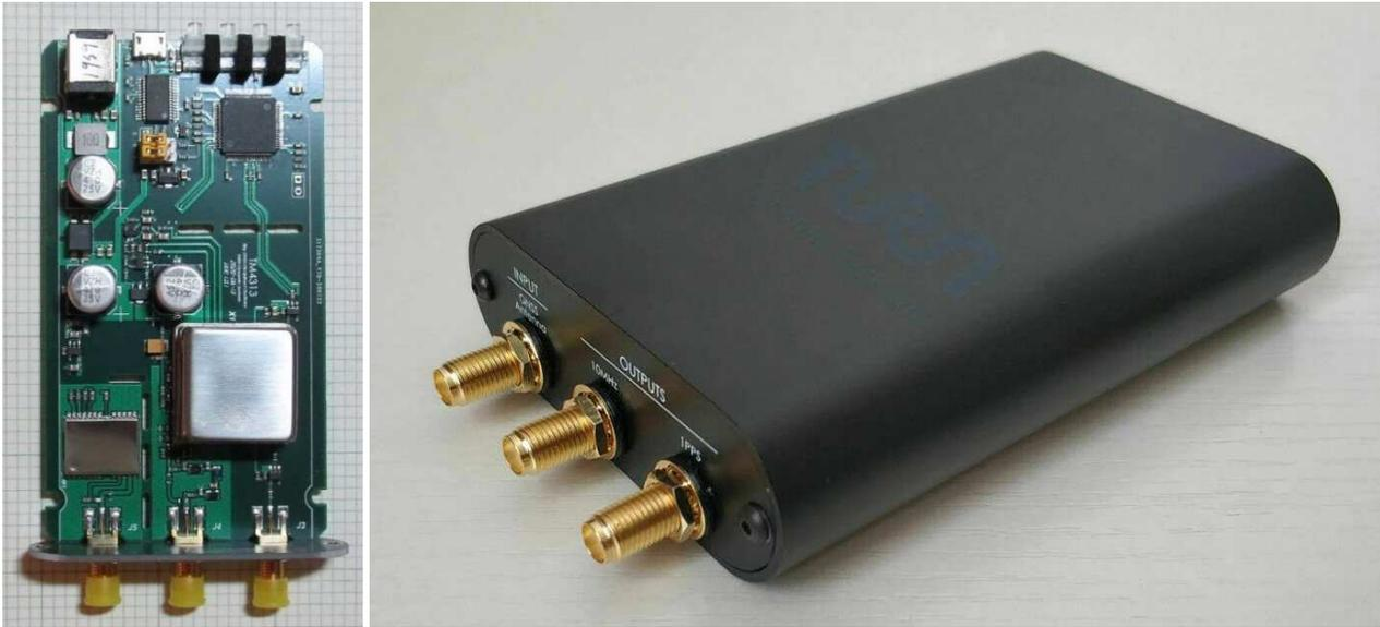
Figure 5.a ~ Left: System PCB for one of the two units evaluated. The OXCO is the large, square silver can; note the newer appearance than the BG7TBL-D and SatTime (before replacement). The 10 MHz and 1 PPS outputs and antenna input are at the bottom, and the dc power jack, Micro-USB connector and LED indicators are at the top of the image. Right: View of the output and antenna input panel. The outputs are 10 MHz sinewave and 1 PPS.
