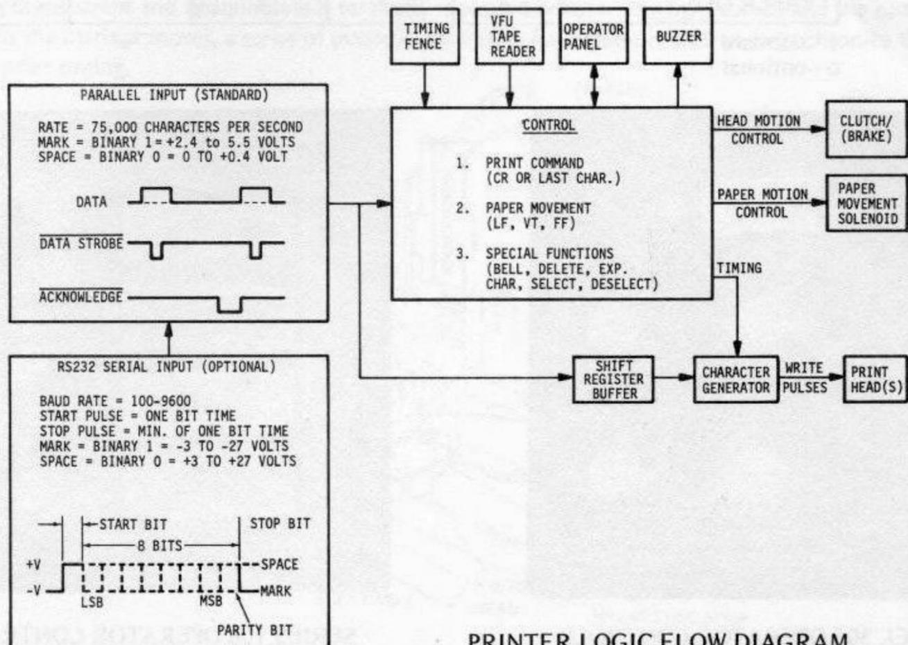
PRINTER LOGIC FLOW DIAGRAM
