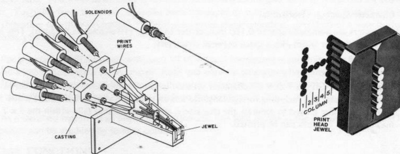
Printing action is initiated when the input buffer is filled or a Carriage Return code is received. The print head then sweeps across the page at a constant rate until the last character in the buffer is printed or the print head carriage reaches the limit switch. As an option in the 306 and 101AL, any paper movement command (FF, VT, or LF) can also initiate a printing action.
