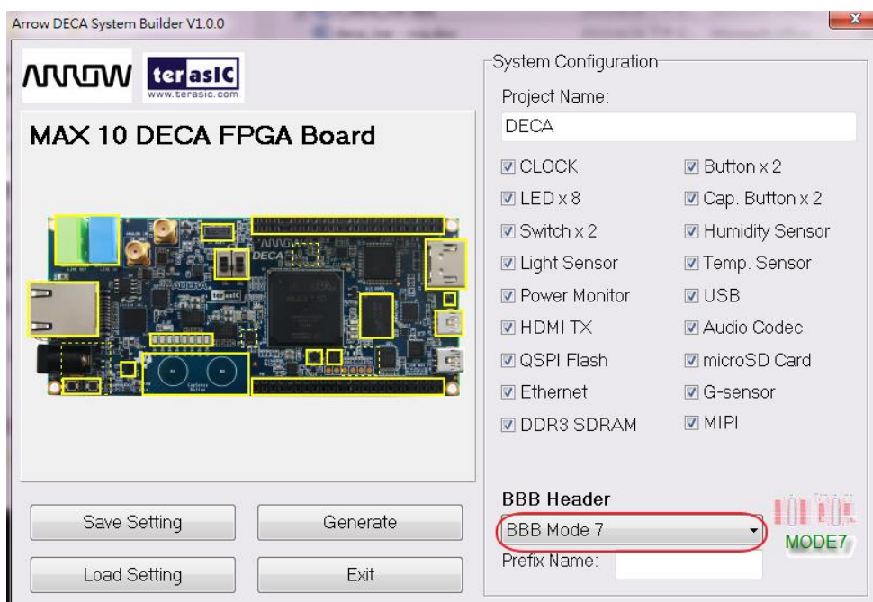
Figure 4-5 GPIO expansion group
