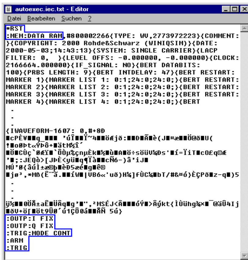
Fig. 7 shows the altered content of the waveform file. The altered IEC/IEEE-bus commands are surrounded by boxes to highlight their location in the file. The content of the file has been condensed in order to show how the IEC/IEEE-bus command sequence is arranged in the file.
